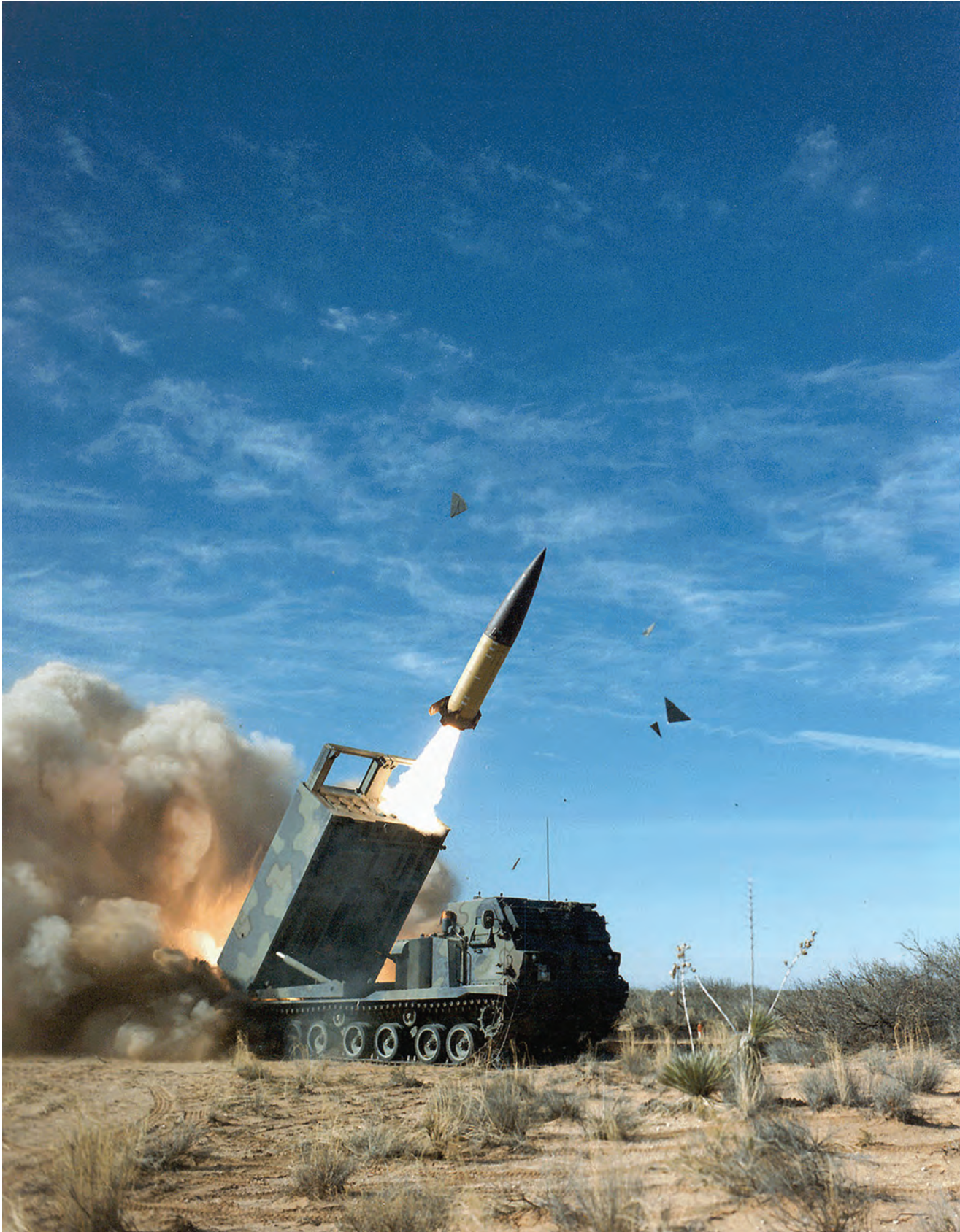
The Multiple Launch Rocket System (MLRS) can launch a mix of offensive munitions, including the Army Tactical Missile System (ATACMS) and other rockets. Source: U.S. Army.
